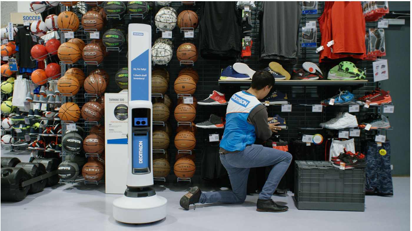
Tally alerts store associates to out-of-stock items so they can quickly refill empty shelves.
